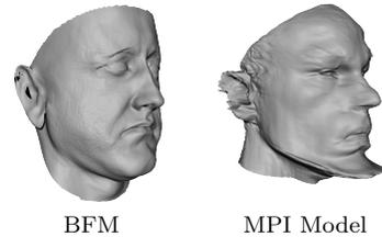
Figure 1. Correspondence artifacts caused by the surface parametrization occur especially for larger values of model coefficients. Rendering the MPI model (right) and the BFM (left) with the same coefficient vector ( $c_i \sim \mathcal{N}(0, (2.5)^2)$ ) shows that the new BFM displays less artifacts.
