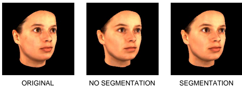
Fig. 4. In order to recover more of the characteristics of a test image (left), after optimizing model parameters for the whole face (center), separate sets of parameters are optimized for different facial subregions independently (right). As subregions, we used eyes, nose, mouth and the surrounding area. Improvements can be seen in the reconstructed shape of lips and eyes.
