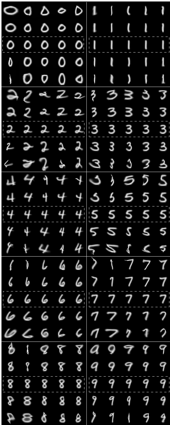
Figure 4: For each of the 10 digits the figure shows the first five shape eigenvectors (left to right) of the model (obtained from 250 prototypical digits). Each column display how each shape eigenvector changes relative to the average digit (in dashed box). The range of the coefficient ranges from +5 (top) to -5 standard deviations (bottom) of each eigenvector.
