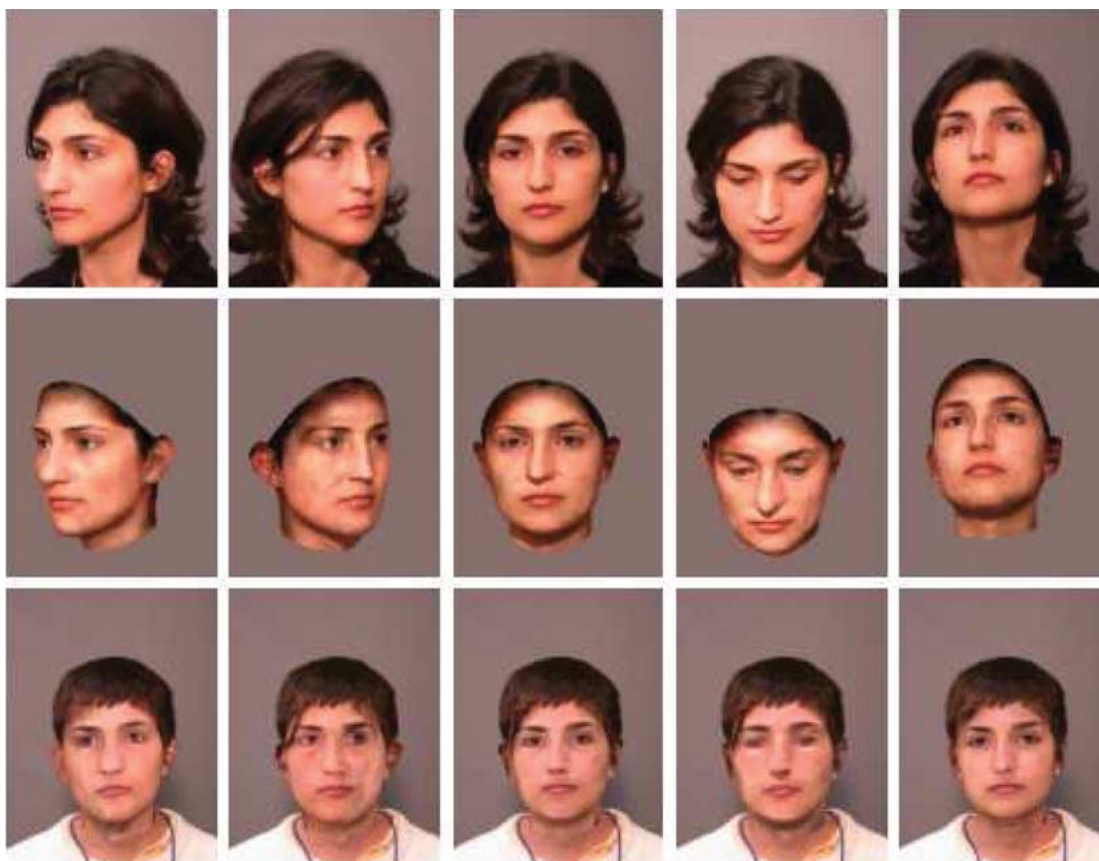
Fig. 12. 3DMM is fit to the original images (top row). Renderings of the fitting result are shown in the middle row. Mapping the texture of visible face regions on the surface and rendering it with a standard background produce virtual front views (bottom row). This figure was first published in the face Recognition Vendor Test 2002 [31].
