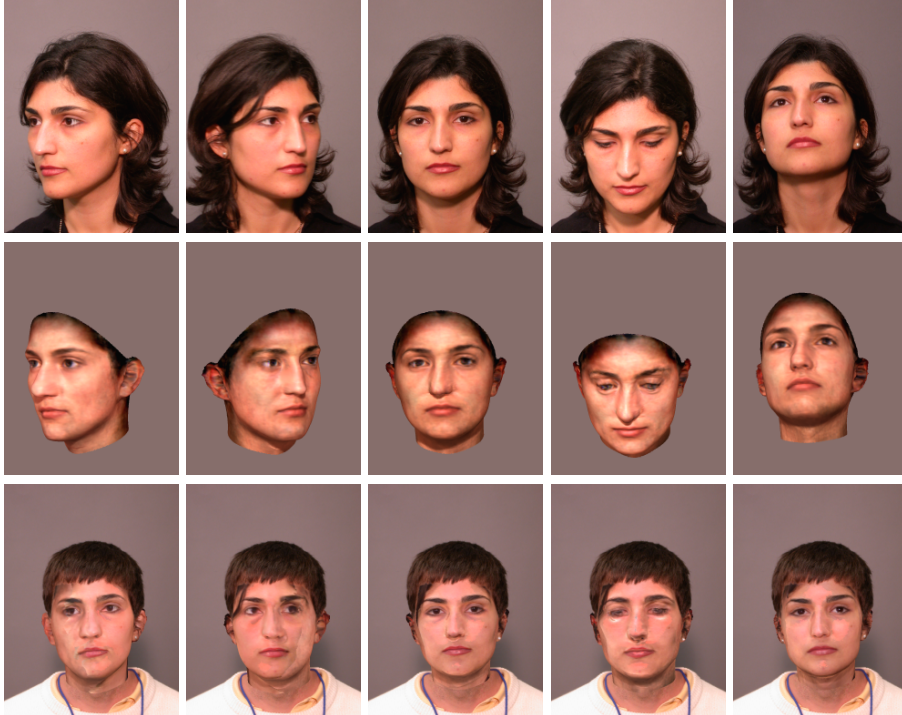
Figure 4: From the original images (top row), we recover 3D shape (second row), by finding an optimal linear combination of example faces, and redraw the faces in frontal pose into a standard background (bottom row). In Section 4.1, the original front view (top, center) was used in the gallery, and the four non-frontal originals (top) and all five transformed views (bottom) were in the nine probe sets, respectively. The frontal-to-frontal mapping served as a baseline test (bottom row, center).
