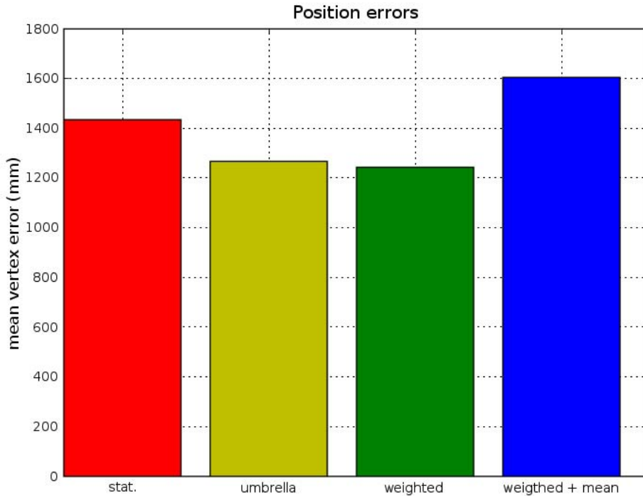
Figure 6. Comparison of the error in generalizing the vertices positions, for the different reconstruction methods: statistical ( 1.43 \cdot 10^3 ), Poisson using the umbrella operator ( 1.27 \cdot 10^3 ), Poisson using the operator described in section 4.2 ( 1.24 \cdot 10^3 ), and the Poisson using the latter operator but the mean as guidance ( 1.61 \cdot 10^3 ).
