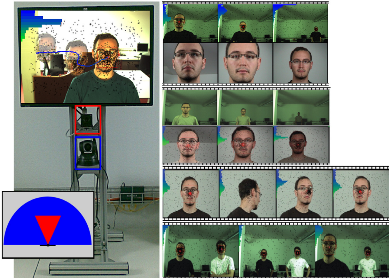
Fig. 6. Our active dual camera system (left) demonstrates robust CCT in three dimensions (right), even for short occlusion of the object and for multiple objects (right, 5th and 6th row).
