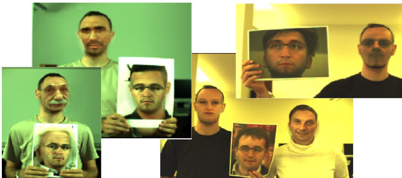
Fig. 8. HCI application FaceSwap applying 3D CCT. FaceSwap is an enjoyable eye-capture by touching questions from the field of perception psychology. The performance of the 3D CCT is demonstrated by tracking multiple persons and swapping their faces or with faces on photographs.
