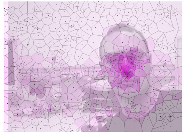
Fig. 5. The computational complexity is twice contracted to regions with high probability to contain objects of interest. For difficult to discriminate feature space regions (pink) more operations per measurement location (W-RVM) and a higher sample density (Condensation) are used, than for homogenous areas (white). (For interpretation of the references to color in this figure legend, the reader is referred to the web version of this article.)
