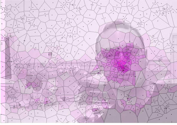
Figure 5: The computational complexity is twice contracted to regions with high probability to contain objects of interest. For difficult to discriminate feature space regions ( pink ) more operations per measurement location (W-RVM) and a higher sample density (Condensation) are used, than for homogenous areas ( white ).
