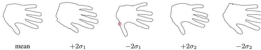
Fig. 4. The first two principal components of the model. No artifacts are visible, despite the large number of artifacts in the data set. At segment boundaries, small discontinuities can appear (red circle), when the segment is reconstructed from limited data.
